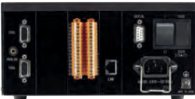
CONTROLLER BACK PANEL 1. Ethernet connector (option) 2. I/O terminal board 3. Tool connector 1 4. Tool connector 2
