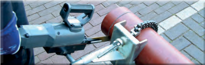
Always use the tube spanner and chain for fixation of the tool!
