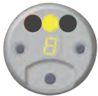
FLASHING YELLOW low battery warning
