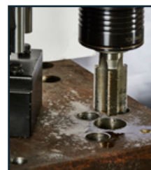
Tapping capacity M44 See pages 42-43 for solutions
