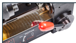
Safety conscious separate magnet and motor switch gear - prevents accidental start up
