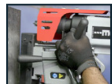
Self-correcting slide rails
