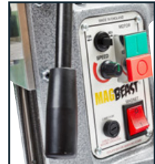
Variable speed & forward/reverse simple control panel
