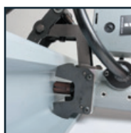
Featuring clamp and Turbo rail cutter
